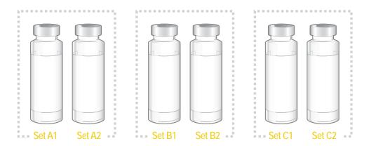
**Step 3.** Now, by use of IV transfer tubing sets and vented needles or spikes, transfer approximately 25 ml into each of the 6 empty 50-mL vials from the 3 test media vials provided.
